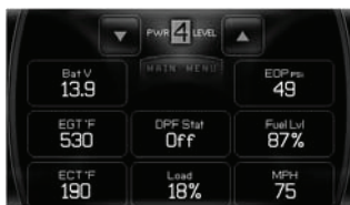
Monitors vehicle vitals by displaying up to 8 different parameters at a time
